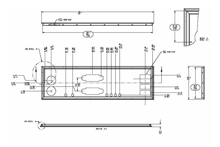
Figure 12. sku 1 Pedestal mount I/O shield mechanical drawing
